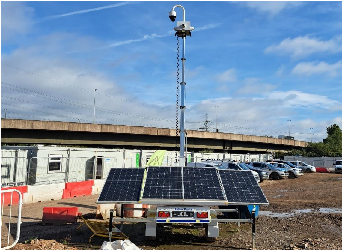
Figure 30 Washwood Heath (Sublot 4) solar powered security system.
