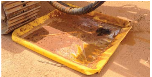
Temporary drip tray (bund) for a leaking hose.
