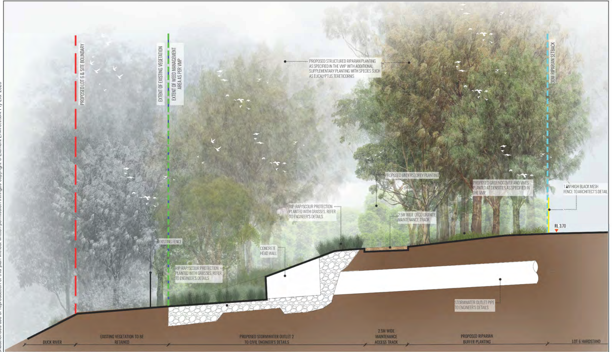
Figure 3.22 Typical section through riparian corridor showing stormwater outfall
