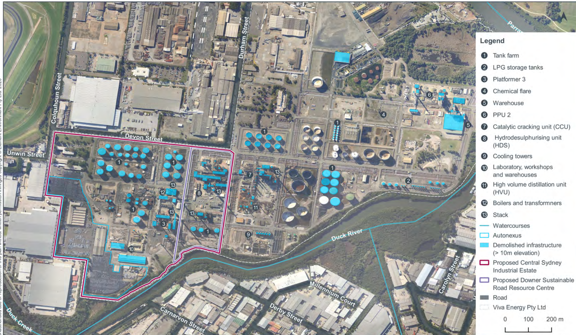
Figure 2.1 Demolished Clyde Refinery infrastructure (>10m height)
