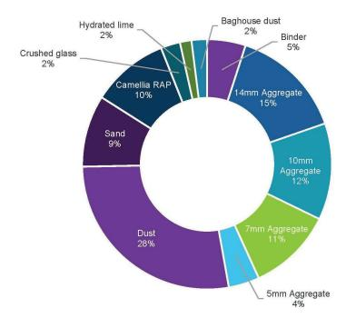
Table 5: Materials used for manufacturing for Mix AC14H A15E, AC14H AR450, AC14 AR450, AC20 AR450 A and AC20 AR450 (per tonne of asphalt)
